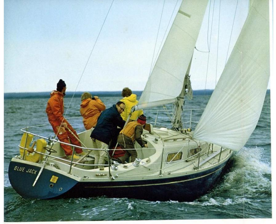
The Albin Ballad has been specially designed for competing on equal terms in the half ton class. She is very easy to sail and handle. Great trouble having been taken to ensure that the boat is beautifully balanced with the centre of the hull's resistance correctly situated in relationship to the sails centre of effort.
