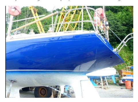
With the top sides and deck re-sprayed using Awlgrip, the boat was starting to look the part. During the summer of 2011, we sailed to Brittany and Isles of Scilly spending most of our spare time picking of masking tape which was left on the stainless and hull by the sprayer. This gave us time to think about the more structural parts of the boat, which needed addressing.
