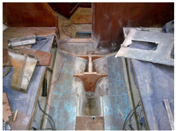
I then used M10 machine screws to tap and glue the Selden mast foot into the oak pad. This was now solid and ready for the mast to be stepped. The whole job cost me 8 hours of my time and £300 for the composite mast step. This is a lot less then the £1500 quoted by a boat yard to do the job.
