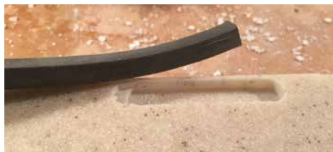
A channel has been routed in the flange
