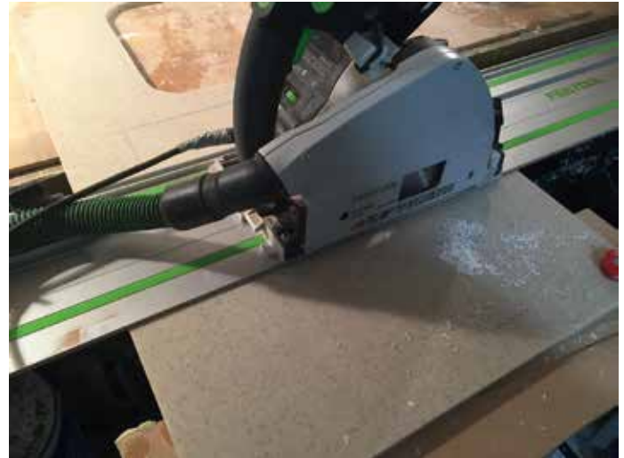
Enter stage right the awesome (if mildly terrifying) Festool circular plunge saw with its guide rail
