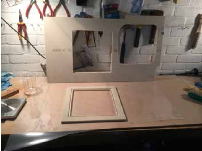
Lining up the flange with the worktop
