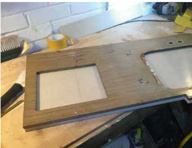
It's time to reattach your template in order to start routing the edge
